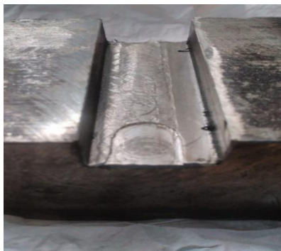
Figure 4 Die grooved for resembling crack
