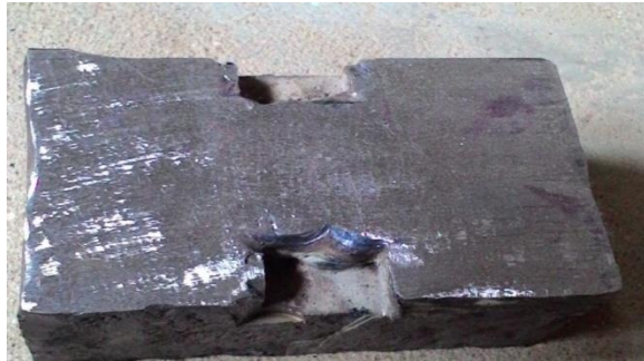
Figure 6 Die after reinforcement welding.
