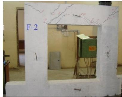
Figure 5. Failure Pattern of Frame (F-2)
