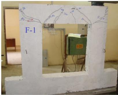
Figure 4. Failure Pattern of Frame (F-1)
