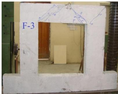
Figure 6. Failure Pattern of Frame (F-3)
