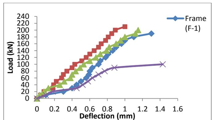
**Figure 3.** Load-deflection Curves of Tested Frames
