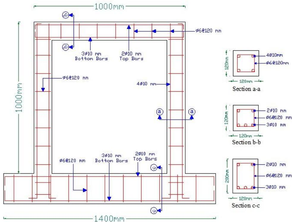
Figure 1. Details of Tested Frames
