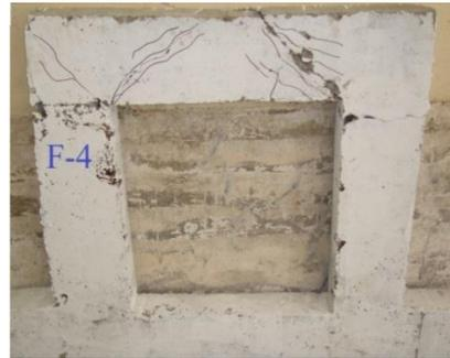
Figure 7. Failure Pattern of Frame (F-4)
