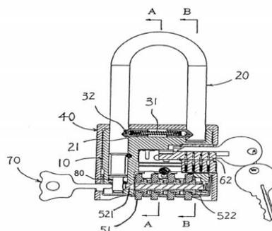
**Figure 4: Combination Padlock with Double Key**
