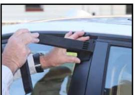
**Step one:** Use the tool to open a gap into the vehicle, as shown in these two photos.
