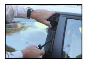
Then operate the inside power door lock control with the tool. The power door lock switch on most BMW models is located on or near the center console. On later model vehicles, it is located on the dash between the air conditioning ducts as shown in the photos. When you press the power door lock button, be sure to listen for the power door lock motor to cycle inside the door; if you don't hear the motor, you have not operated the power locks.
