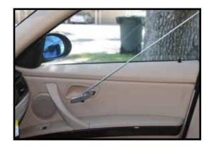
Either on the same side of the car that you are working on, as shown, or on the opposite side of the car. When the inside lock control button pops up, you will have disengaged the deadlock system.
