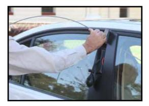
**Step two:** Re-bend the tool as shown so that you can attack the inside door handle.
