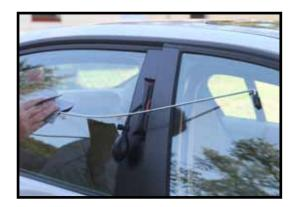
In order to push the power lock button, you will have to put a "reverse bend" in the long reach tool, so that the flat part of the tip is squarely against the power lock button. (See photos)
