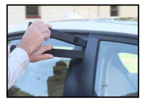
The type-3 deadlock system, which is the most common, can be defeated in a three step operation using a flexible long reach tool.
